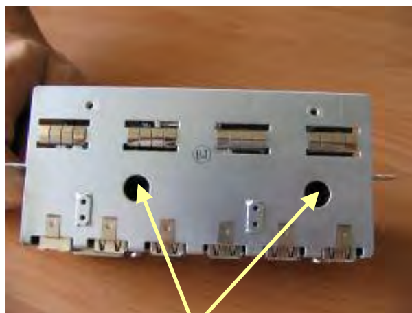
Two M3×6 Screws in Holes
